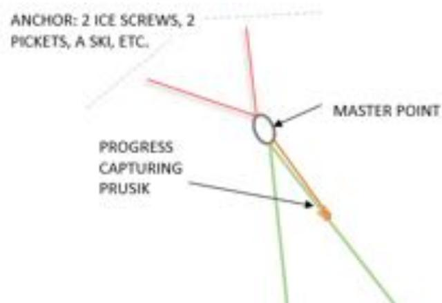
Note that if you have a microtraxion, placing it at the master point is an excellent backup to the progress capturing prusik, but isn't necessary. Next, tie a prusik hitch a few meters down the main line towards the climber. Attach a carabiner on the end of the prusik, clipping in the rescue line (the unweighted rope of the other side of the master point).
