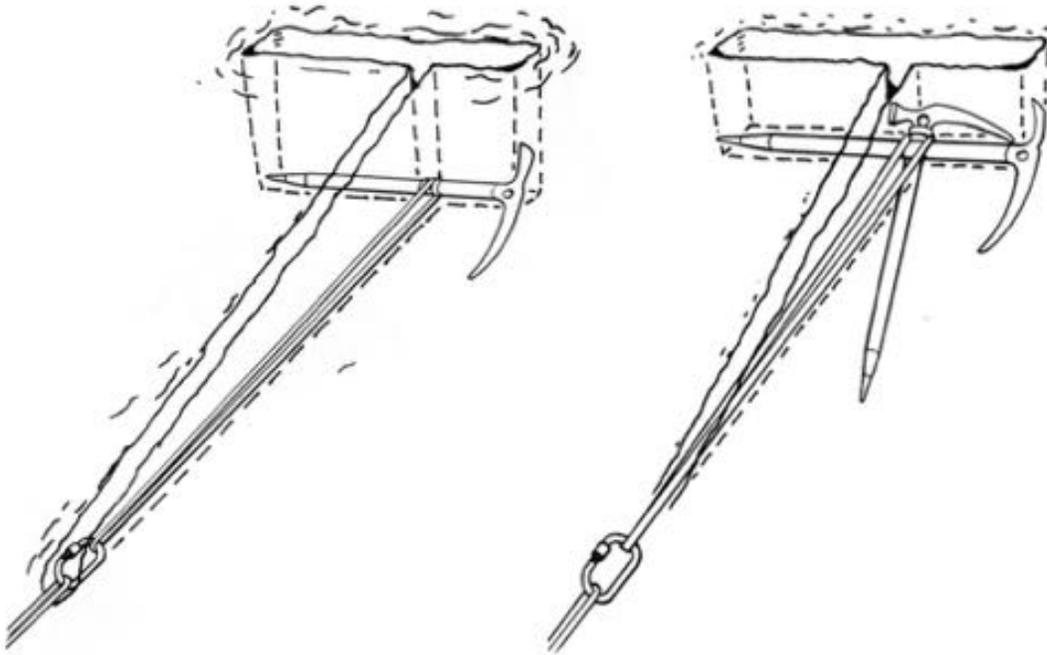
FIGURE 5 - TWO TYPE OF T-SLOT ANCHORS USING ICE AXES (OFFGRIDWEB.COM)
