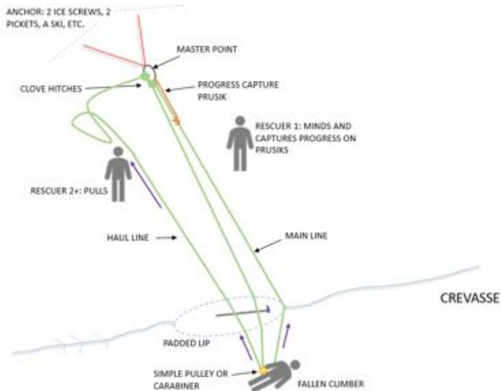
This system has another underrated advantage: the climber and their pack can be hauled upwards in two separate hauls if they are too heavy to haul together. So while the advantage is only 2:1, the weight of the haul can be significantly reduced. However, should this still not be enough mechanical advantage, the 2:1 drop loop sets the scene well for a third option.
