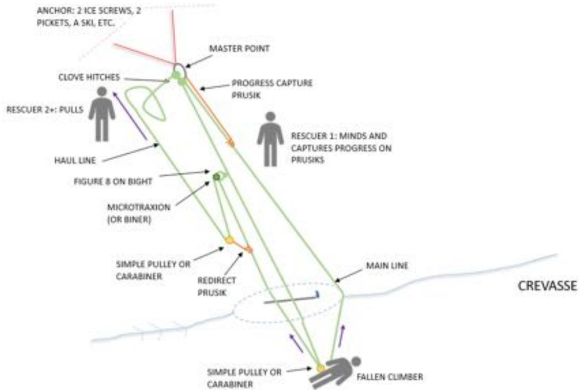
Similarly to the 2:1 drop loop, this system is most effective if the climber is conscious and can clip the carabiner into their belay loop. If the 3:1 Z-pulley is out of the question and a drop loop must be used, it is worth knowing how to rappel down to the climber to clip them in. This is also a useful technique in case the fallen climber needs immediate first aid (i.e. to stop a serious bleed). However, due to the tight G1 schedule, this is a technique that is generally reserved for G2 field.
